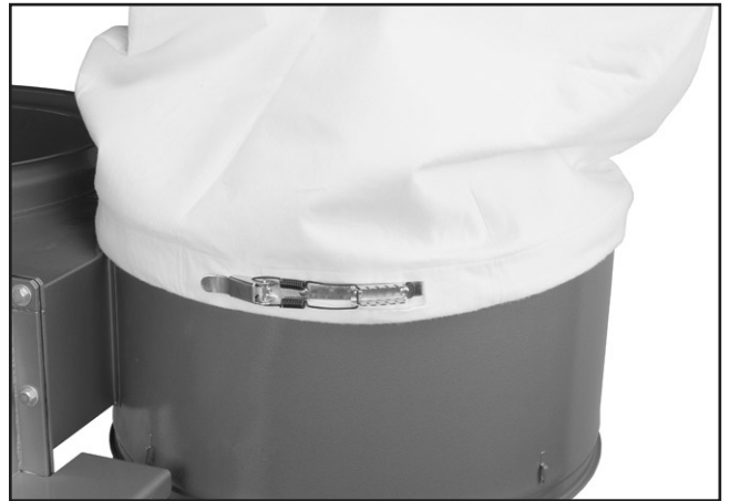
Figure 9. Fitting bag onto collector.
